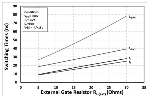
Figure 26. Switching Times vs.  $R_{G(\text{ext})}$
