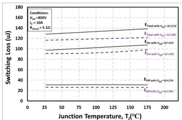
Figure 25. Clamped Inductive Switching Energy vs. Temperature
