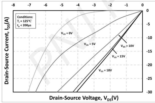
Figure 17. 3rd Quadrant Characteristic at  $125^\circ\text{C}$
