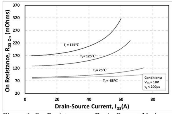
Figure 6. On-Resistance vs. Drain Current Various Temperatures
