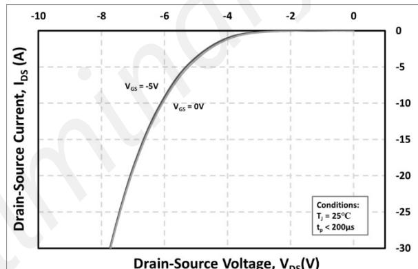
Figure 10. Body Diode Characteristic at  $25^\circ C$
