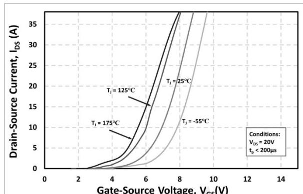
Figure 8. Transfer Characteristic for Various Junction Temperatures
