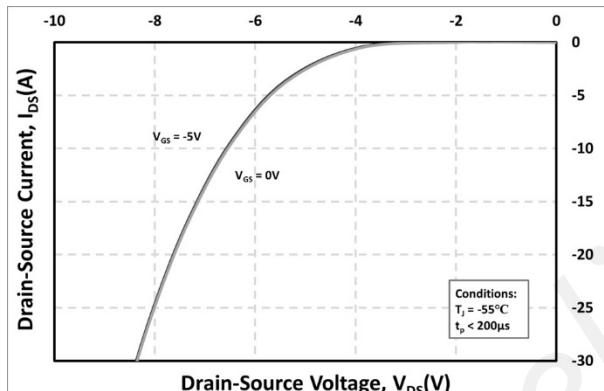
Figure 9. Body Diode Characteristic at  $-55^\circ C$
