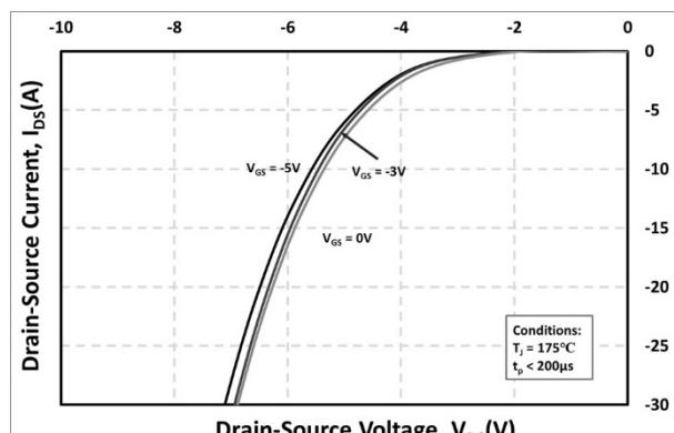
Figure 12. Body Diode Characteristic at  $175^\circ C$
