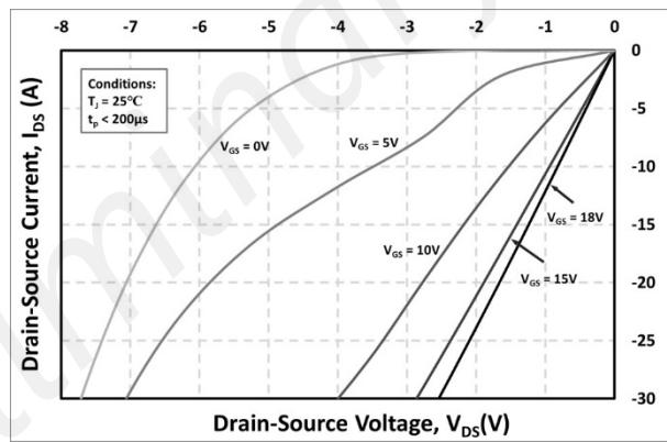
Figure 16. 3rd Quadrant Characteristic at  $25^\circ\text{C}$
