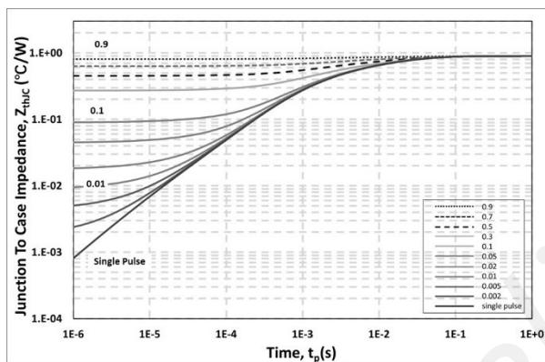
Figure 27. Transient Thermal Impedance (Junction - Case)
