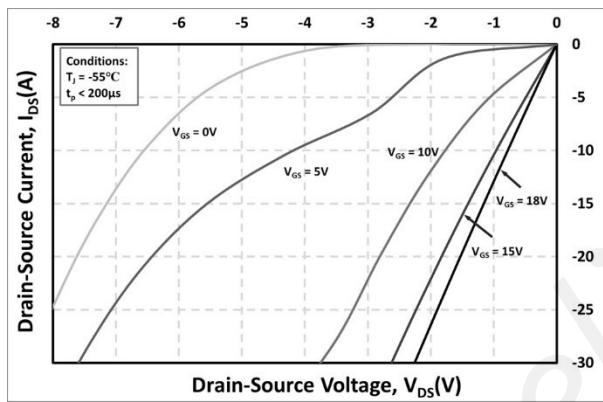
Figure 15. 3rd Quadrant Characteristic at  $-55^\circ\text{C}$
