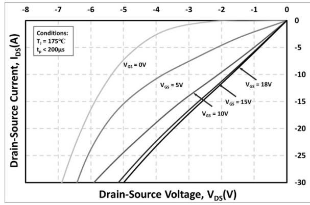
Figure 18. 3rd Quadrant Characteristic at  $175^\circ\text{C}$
